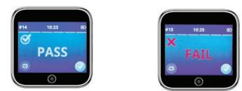
**Pass/Fail Level** -Used to select the levels for "Pass" and "Fail". If the "Pass" and "Fail" level are next to each other then you will not see "Warn".
