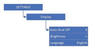
Auto Shut Off sets the time the unit will stay on without a keypress. Press Execute to select time.
