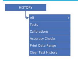
The History menu is where all tests, calibrations and accuracy checks are stored. The LX9 can store up to 10,000 tests in memory. Any test, calibration or accuracy check in memory can be viewed or printed.
