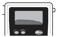
As the subject blows into the mouthpiece, the FC10 will show a graph of the breath flow on the display, as well as showing the amount of liters. Liters are shown in the upper left corner.
