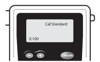
Use the **+ or -** button to change the number to the BAC level of standard you will be calibrating to. It should be the same as on the bottle of certified solution or as your altitude corrected standard, if using a dry gas tank. (See p. 14)
