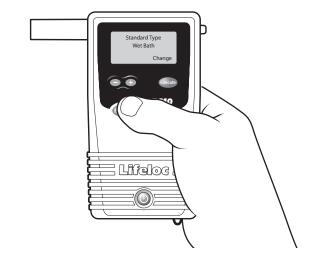
Press the **Function** button to save settings. Momentarily press **Power** to return to the testing mode.
