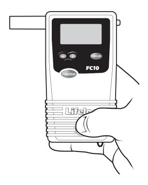
Press and hold the Power button on the bottom of the front of the unit until it beeps. The FC10 performs an automatic internal diagnostics check.
